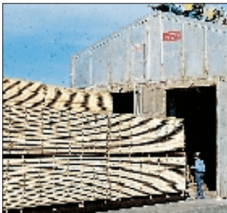
Properly drying and conditioning Southern Pine in a kiln helps reduce warping, splits and checks.
