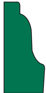
# 210 Shingle Mould 11/16 x 1-5/8
