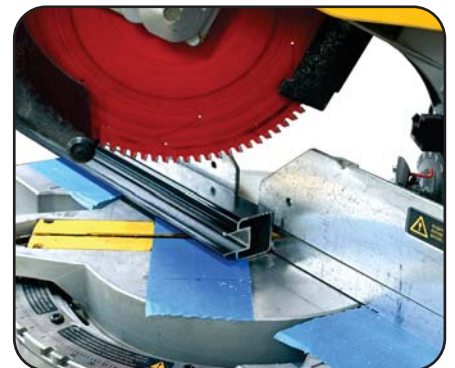
(6) Cut Top Rail Cut the Series 250 top rail at the angle of the stairs using a high-tooth count metal cutting saw. Paint the cut ends.
