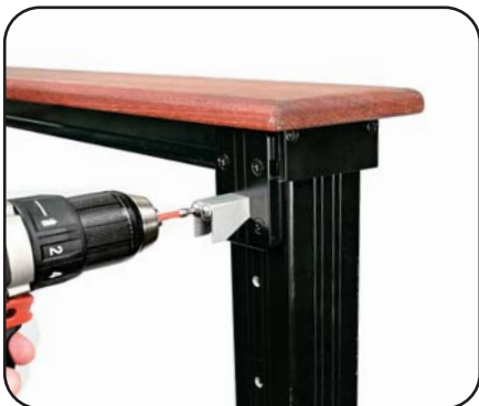
(5) Attach RCB to End Plate Attach the RCB to the end plate bracket. Attaches with 2 ea. screws using #2 square drive.
