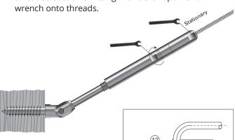
14. Tension all cables in sequence, beginning with the center cables, moving up and down toward the top and bottom. As you tension each cable, give it a sharp pull downward mid-span to help set the wedges, then retension as necessary in the same sequence.
