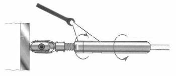
12. Tension in sequence, beginning with the outside cables and moving back and forth toward the center. Finished cables should be tensioned to have only 1/4" of play when finger-pulled.
