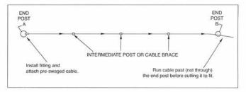
If you are bending cable across a landing with wood posts, you will want to insert a Post-Protector Tube (order CS-TUBE-6 separately from Accessories) into the wood post where the cable angles out of the post. Drill a 1/4" hole 1-1/2" deep straight into the post to receive the CS-Tube.
