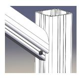
RFX100/250 Infill Snip RCB to allow Infill to be snapped on for a finished look. Install prior to tensioning the cables.
