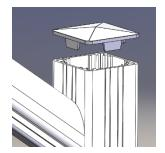
Install Post Cap Install post cap. Use adhesive to secure cap to post.
