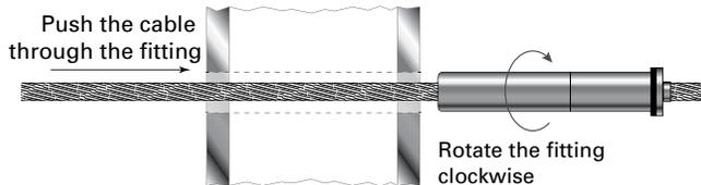
3. Push the Pull-Lock fitting along the cable and firmly into the hole in your post. While holding the Pull-Lock fitting against the end post, pull the bare end of the cable to remove as much slack in the cable as possible.
