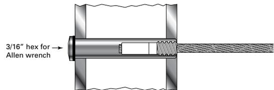
The swaging stud will be pulled into the Receiver by rotating the Receiver clockwise.
