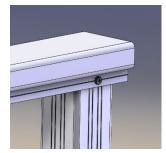
Attaching to End Post Rail slides over top of post and attaches with 2 each screws..
