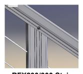
RFX200/300 Stair Intermediate Post Cut post at the angle of the stairs. Rail slides over top of post and attaches with 2 each screws. 1 screw per side.
