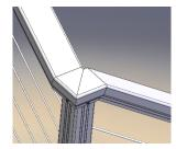
Stair Splice – Application 2 Example of rail mitered down the stairs in with a 90 degree turn.
