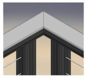
Angled Splice Splices are also used to attach corner rails. Angles include 45, 90 and custom degrees.
