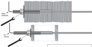
Tension all cables to desired amount in sequence, beginning with the top and bottom cables, moving up and down toward the center.
