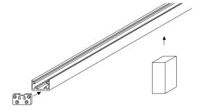
**c.** Locate crush block(s) provided to the bottom Aluminum Rail Reinforcement, with spacing no greater than 36" from the end, or between Crush Blocks.
