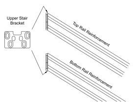
Attach an upper stair bracket to the angle cut end of the top rail reinforcement, with the bracket flush with the top of the reinforcement, using four *rail bracket screw* (A). Attach an upper stair bracket to the angle cut end of the bottom rail reinforcement, with the bracket flush with the bottom of the reinforcement, using four *rail bracket screw* (A). Lubricate the threads with soap to avoid binding and use a clutch type drill to avoid stripping screws.
