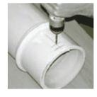
STEP 11: Mark and drill clearance holes on the top and bottom of the column to accommodate bolts for the 1 1/2" L-brackets. (L-brackets sold separately.)
