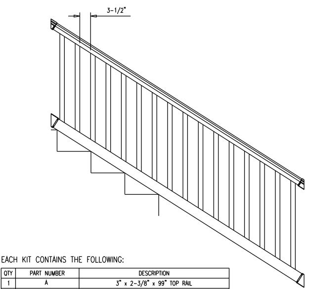
OTY PART NUMBER 2-1/4" x 3-1/4" x 99-1/2" BOTTOM RAIL В С 3000 TOP RAIL REINFORCEMENT x 96" 1 D 1-1/2" x 1-1/2" x 32-5/8" SQUARE BALUSTER 16 Ε 3" x 2-3/8" TOP STEP BRACKET 2 2-1/4" x 3-1/4" BOTTOM STEP BRACKET 2 16 G MOLDED PLUG 16 Н #10 x 4", SQ. DRIVE, 304SS, TYPE 17, FLAT HD #8 x 1-1/2" PAINTED STAINLESS STEEL SCREW 4
